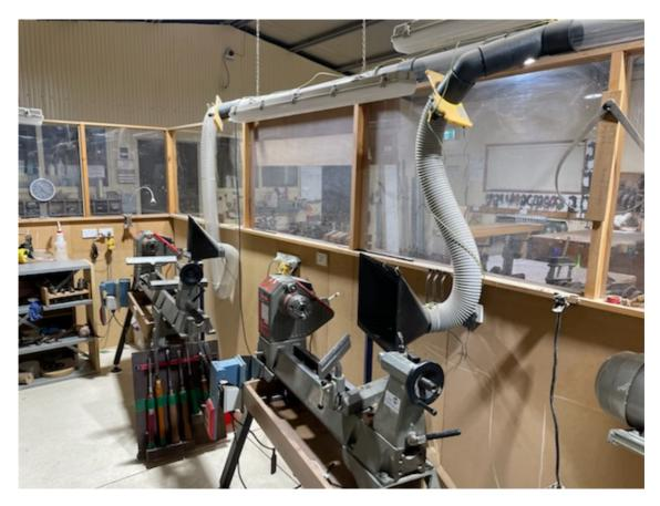
The final electrical connections and testing have been completed for the Dust Extraction system for the Wood Turning and smaller Bandsaws area
