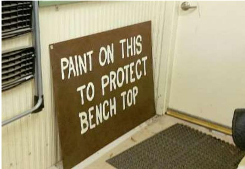
The sheet of masonite outside our tool store is to be placed underneath items being painted to catch all the drips that mess-up the surfaces of our bench tops.
