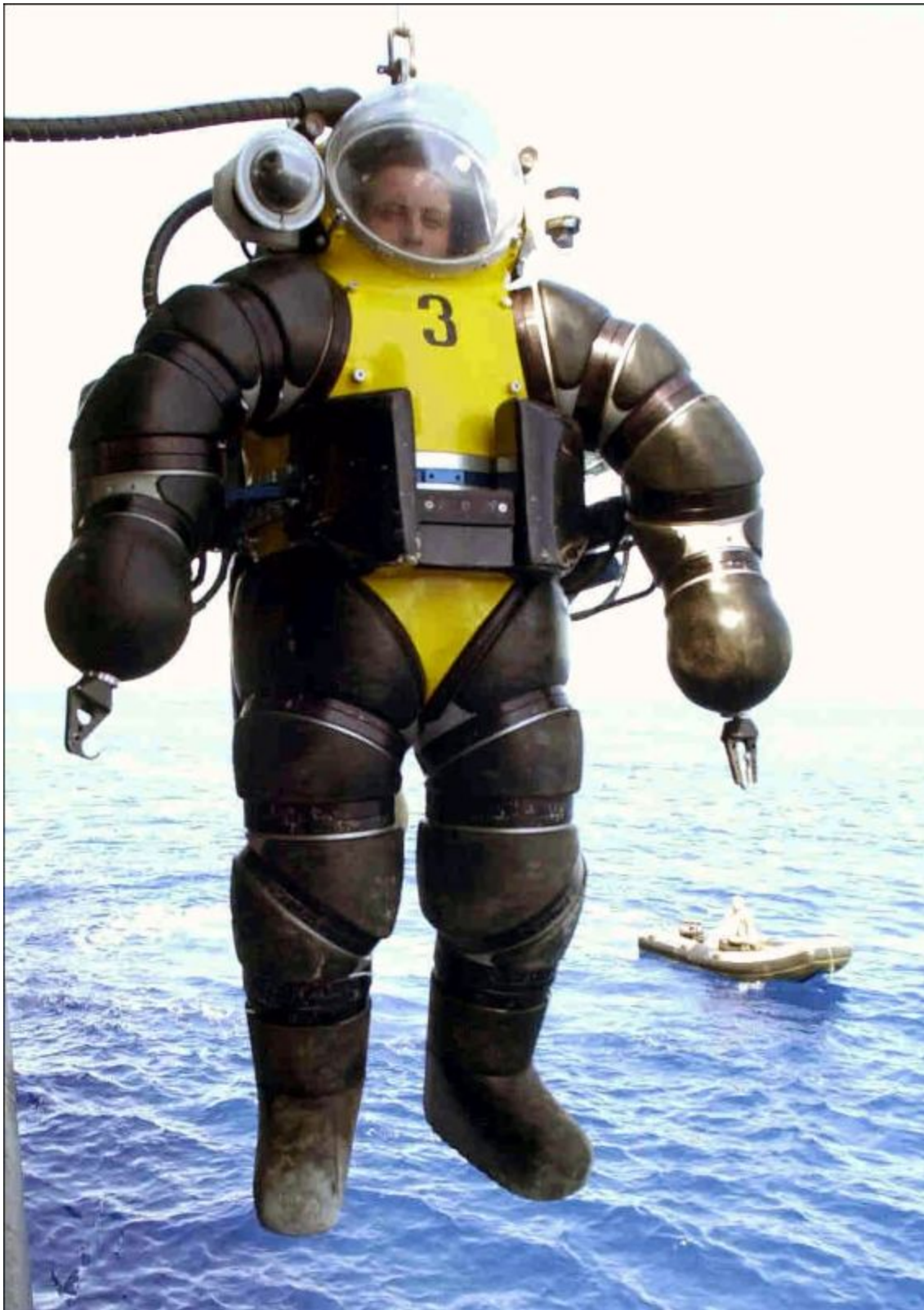
An example of the ADS JIM suit used for underwater construction.
